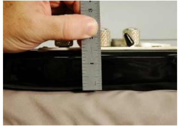
Above: A Squire model with a 1 1/2 inch (38.1mm) thick body. A bridge for anything under 1 3/4 will require a custom cut down block.
